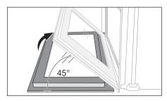
Take hold of the oven door with a hand on each side and pull it away from the oven at an upwards angle (Take care: It is heavy).
